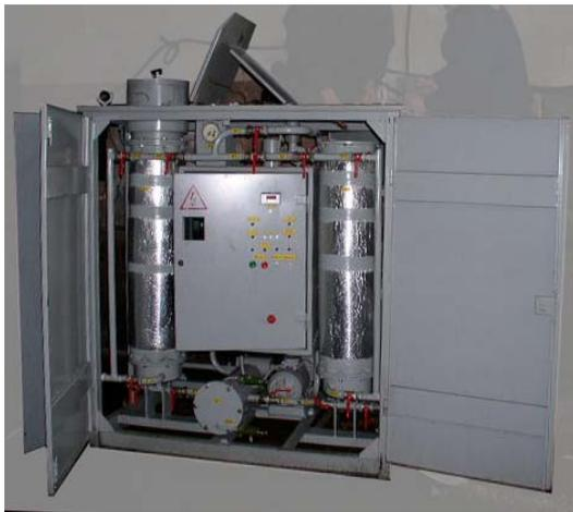
Figure 2 - Industrial equipment for regeneration of transformer oil working on the two-cartridge scheme: one cartridge is used for transformer oil regeneration, second – for adsorbent regeneration. After the regeneration of the adsorbent in the second cartridge, this one substitutes the first one in the scheme of recovery of the transformer oil.
